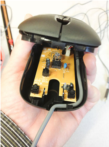
1. Crack open the mouse to liberate the controller
